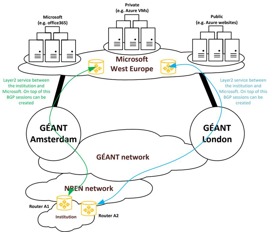
Figure 1: schematic overview of an ExpressRoute connection via GÉANT
